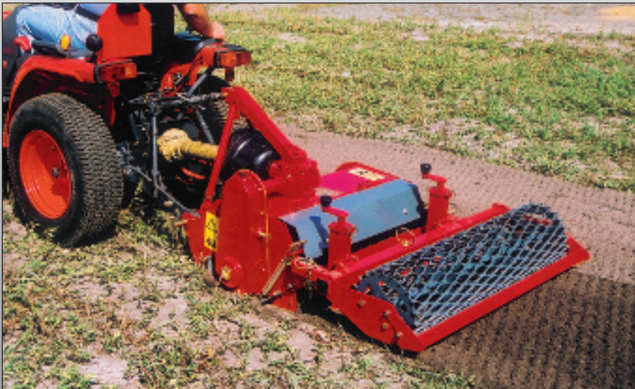
Stony 75 NIV with hydraulic clutch on rotor end
